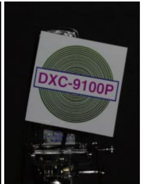
• Progressive Scan CCD - DXC-9100P, frame shutter mode (25 frames, interlaced)
